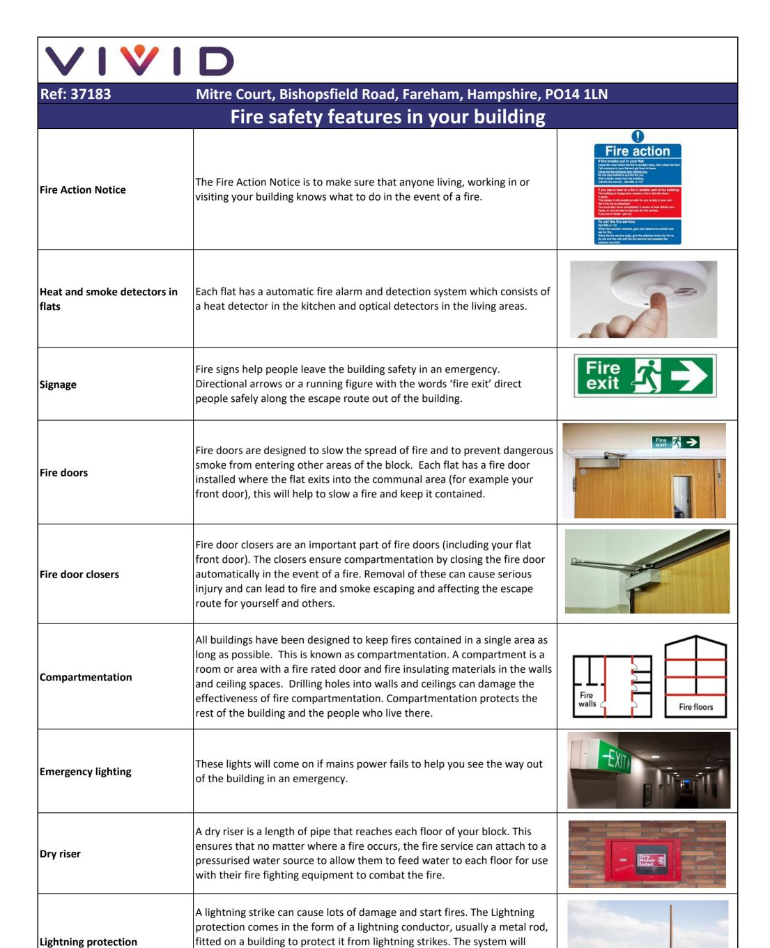
divert a lightning strike to the lightning rod down through a wire allowing it
